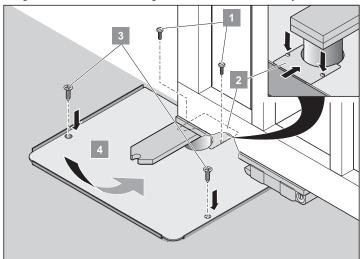
4. Replace the lid (4 + 2) and tighten the screws (3 + 1).
