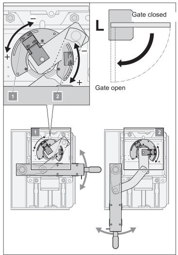
The operator is factory-set to "gate OPEN" (see illustration to the right). The end switches are factory-set for the gate end positions "gate OPEN" and gate CLOSED" to approx. 90°.
