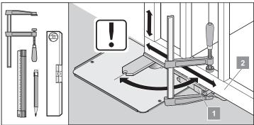
1. Secure the fitting (1) with a vice to the gate (2) and manually open and close the gate to check the fitting's position (1). Adjust the position of the fitting, if required.
