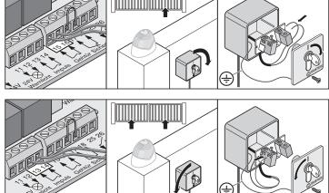
Install key switch box at a suitable location where it can be easily accessed.
