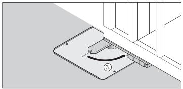
3. Disengage the gate from the gate wing fitting (push against slight resistance).
