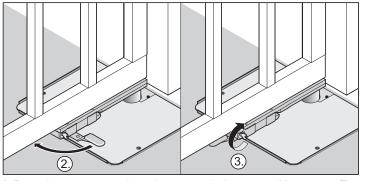
Press the emergency release lever towards the gate until it engages. The gate is locked.  $3\;$  Turn the key by  $90^\circ$  in anticlockwise direction. The emergency release lever is locked.
