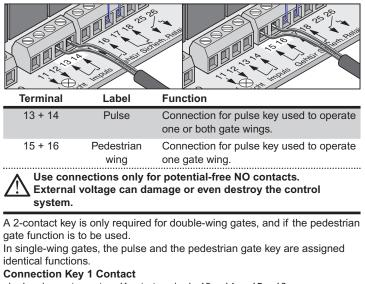
single-wing gate system Key to terminals 13 + 14 or 15 + 16 double-wing gate system Key to terminals 13 + 14
