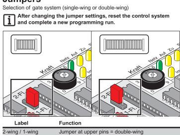
Jumper at upper pins = double-wing Jumper at lower pins = single-wing Jumper not set = single-wing
