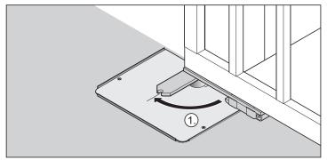
1. Engage the gate in the gate wing fitting (push against slight resistance).
