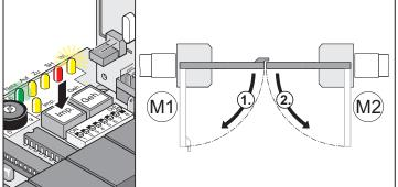
1. Press key (Imp). Gate moves to end position gate "OPEN".
