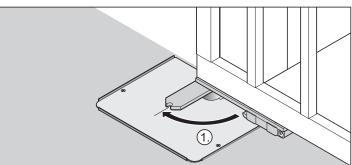
1. Engage the gate in the gate wing fitting (push against slight resistance)
