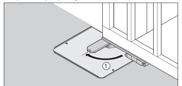
5. Engage the gate in the gate wing fitting (push against slight resistance).
