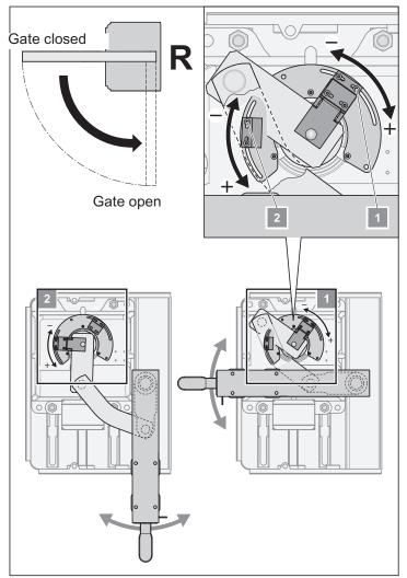
The operator is factory-set to "gate OPEN" (see illustration to the left).The end switches are factory-set for the gate end positions "gate OPEN" and gate CLOSED" to approx. 90°.
